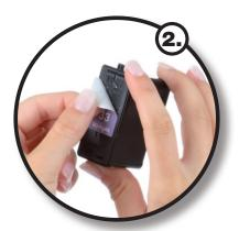
First remove the label from the upper side of the cartridge und bore refilling holes. To do so, use the supplied tool to enlarge the 3 existing openings.
